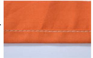
Rolled Hem: narrower version of a standard hem. Typically used in areas where the edge is designed to lift up to reduce weight, such as flutter sleeves and twirly skirts. A rolled hem foot can make this method much easier to sew.
